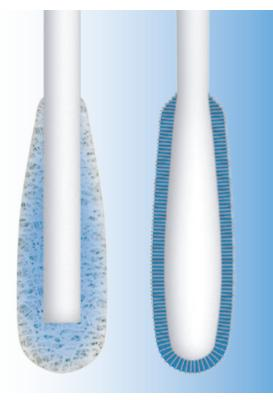
Copan FLOQSwabs™ use short fiber strands which create a thin absorbent layer. The entire sample stays close to the surface for fast and complete elution.
