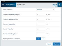
Sample information can be added by scanning sample or reagent barcodes before pipetting.
